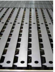
Advanced metal cutting features in the KCAM software allow for control over pierce delays, modulation frequency and a variable air assist.
