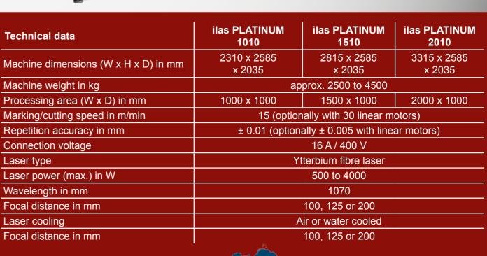
Machine dimensions without operating panel or additional accessories. The laser source and power depend on the individual application.
