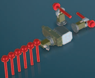
2-finger gripper with 180° rotary module for loading blanks fed in vertically
