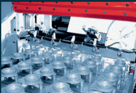
Large storage capacity chain feeding system for loading preformed blanks with the correct orientation.
