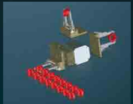
Parallel grippers with 180° rotary module for loading shaft parts (1st and 2nd chucking)
