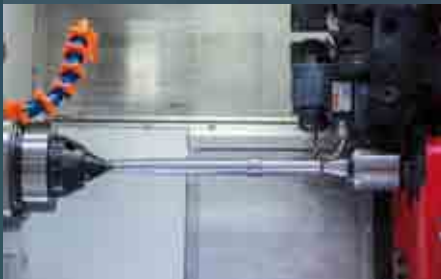
Long workpieces can be clamped between centres and machined along the entire length.
