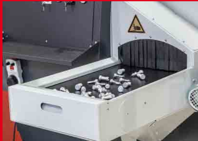
The finished mostly are unloaded with the parts-catcher on to a finished parts are mostly conveyor.
