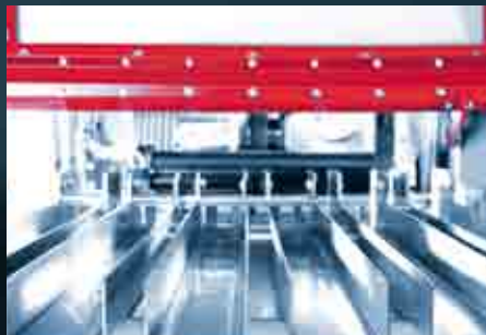
Multiple infeed chutes for loading rotationally-symmetrical blanks. The length of the blanks determines the number of infeed chutes.
