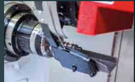
The parts catcher carefully removes finished parts from the work area and takes them to the finished parts container.
