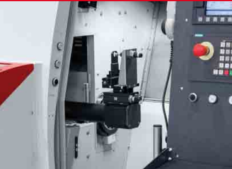
The integrated EMCO Swing LOADER can pick-up the raw part from the feeding system and transfer it through the little door at the side into the machine. There the part is loaded into the chuck against a stop. If needed, the part also can be handled pre-oriented.
