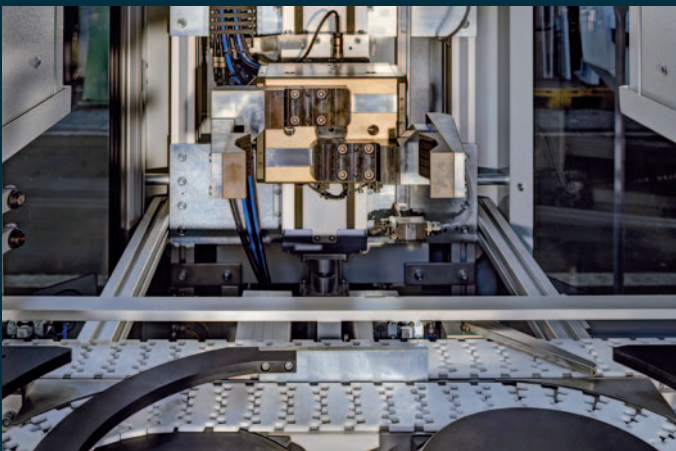
180° workpiece turner with workpiece switch for pallet 1 and pallet 2.
