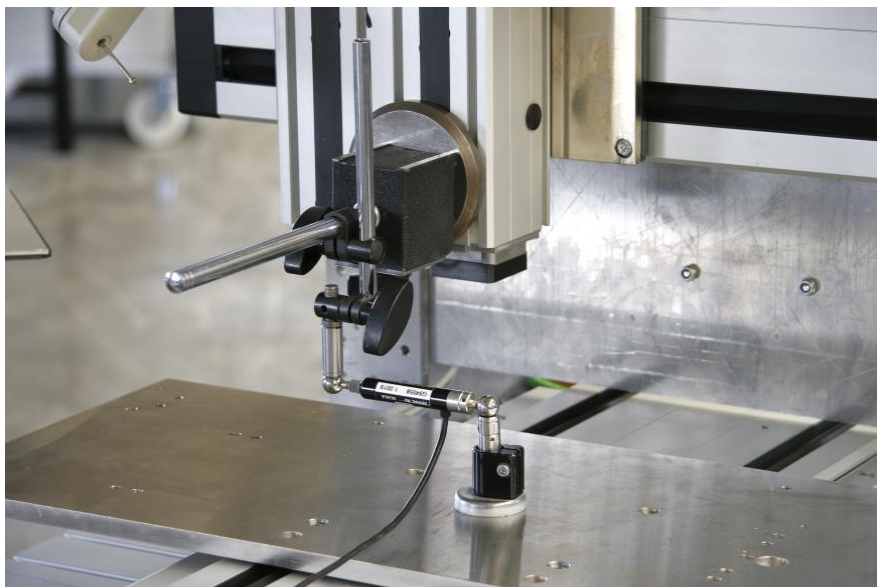
picture: circular form measure with Renishaw QC10
