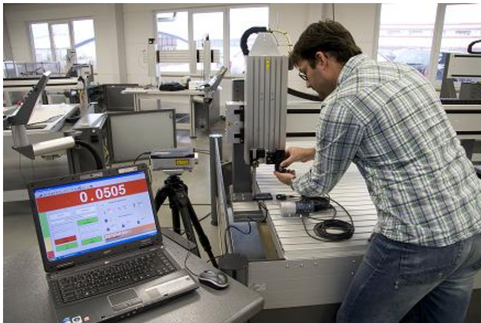
Picture: Laser measurement of an isel base machine in plant Dermbach in Thuringia
