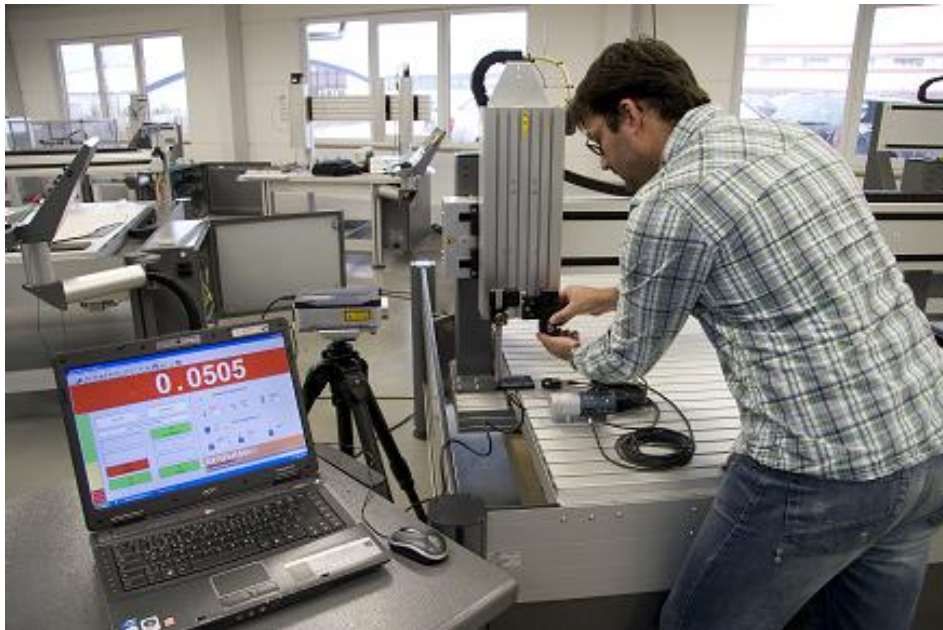
Picture 10: Laser measurement of an isel base machine in plant Dermbach in Thuringia
