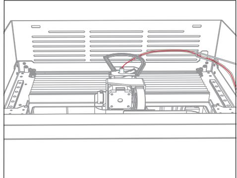
When filament is loaded, insert the end of the filament guide tube unto the Smart Extruder's loading tube and replace and lock the lid of the MakerBot Replicator Z18.
