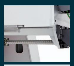
**Y-axis:** The Y-axis has a ram configuration. This design uses long way guides in order to attain the required rigidity. Its high precision is guaranteed by the motor installed direct drive on the screw.
