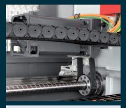
**X-axis:** Equipped with rotating nut ballscrew and fixed screw. The positioning accuracy is guaranteed by the standard linear scale.
