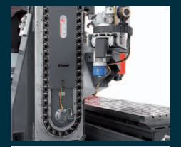
**Tool magazine:** available with turret configuration on 3-, 4- and 5-axis version, or with alongside column configuration on 4- and 5-axis version. Tool change on turret configuration with dual arm grippers at the X-axis limit, with 40 tool stations (optional 80). Tool change on the alongside configuration fast and safe, all along the X-axis and at the extreme limit of the Z- and Y-axis. Up to 120 tool stations. An external tool changer "tower" is available upon request.
