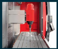
**Milling spindle:** The machine is equipped with a liquid cooled motor spindle with compelling performance specs. At spindle speeds of 15000 rpms, a power rating of 46 kW, and a torque of 170 Nm, the machine is also suited for heavy-duty machining. A motor spindle 18000 rpm is available with HSK A63.
