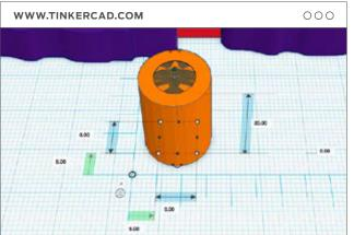
**A. Drag a new box** over from the **basic shapes** menu, then drag a **ruler** to help you out. Click on the cylinder to apply the ruler to it. Change the diameter of the cylinder to 14 mm. B. Make a cylinder hole for the pencil to fit into. Select the first cylinder and duplicate it by pressing ctrl-C then ctrl-V (cmd-C, cmd-V on Mac). Change the size of the second cylinder to 8 mm in diameter and select hole. This will be the cutout for the pencil to fit into.
