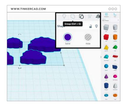
**D. Turn the box into a hole** by selecting the box, then clicking **hole** in the dialogue window near the top right corner.
