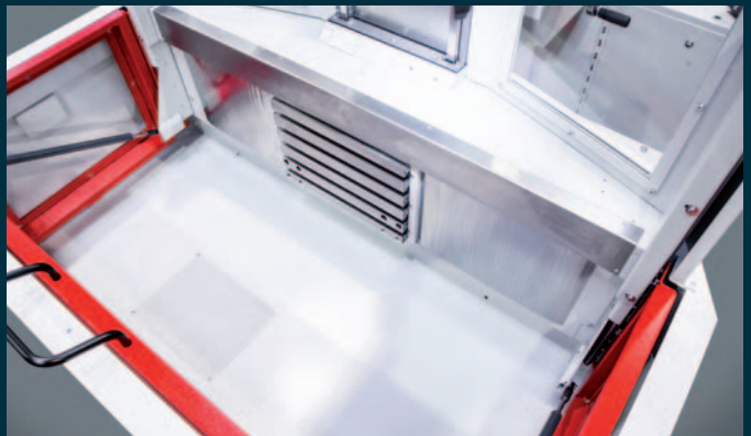
Retractable workspace guard with vertical clamping area.
