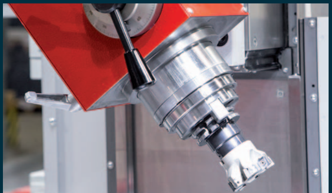
Swivel-mounted vertical milling head with quill for manual drilling operations. Thanks to a swivel range of \pm 90^\circ , even difficult machining can be performed easily.
