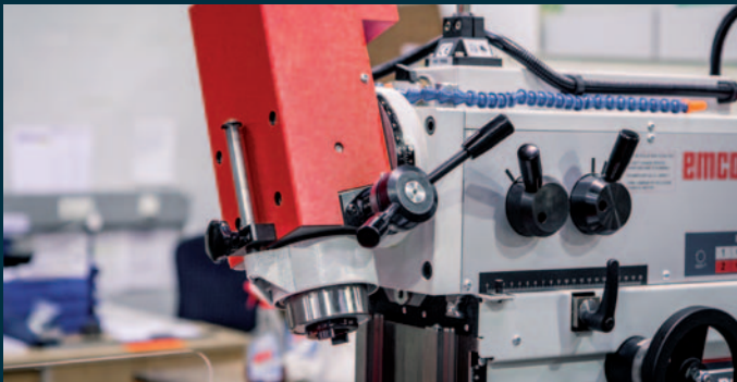
Vertical milling head. Vertical milling head with DIN 2080 SK 30 and clampable 45 mm quill travel. The vertical milling head swivels \pm 90^\circ .
