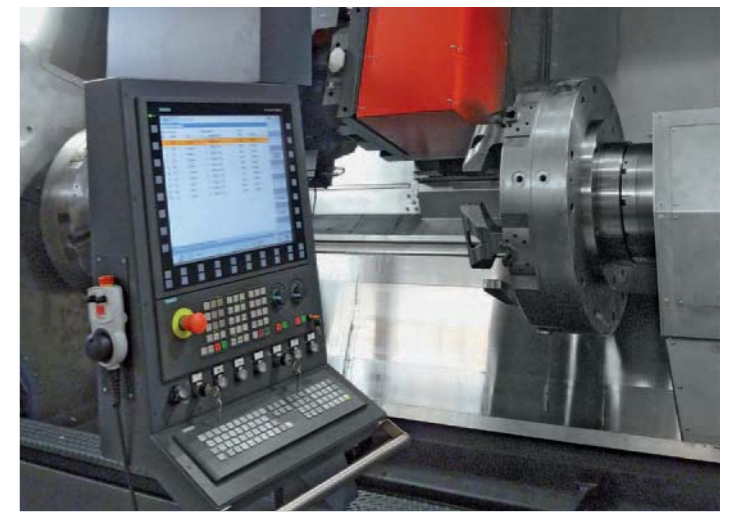
Control system: The machine is equipped with a Siemens 840D sl control. The scope of delivery includes a 22" display with state-of-the-art emcoCONNECT control panel as well as versatile EMCO technology cycles (optional) for easy, dialogue-based programming.
