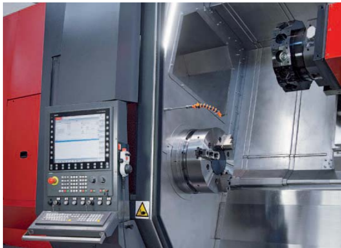
The Maxxturn 200 comes in modular design. Different upgrading levels allow everything from simple turning to the expansion to a turning and milling centre with versatile application possibilities. Different spindle concepts with C-axis and high torque are used.
