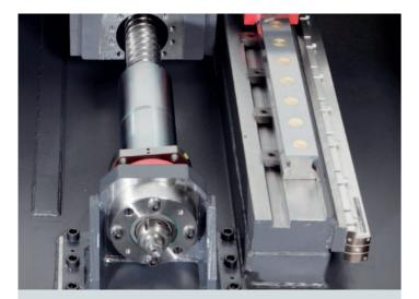
**Glass scales.** Due to its length, the X-axis is always equipped with glass scales. Y- and Z-axis can be equipped with glass scales on demand.
