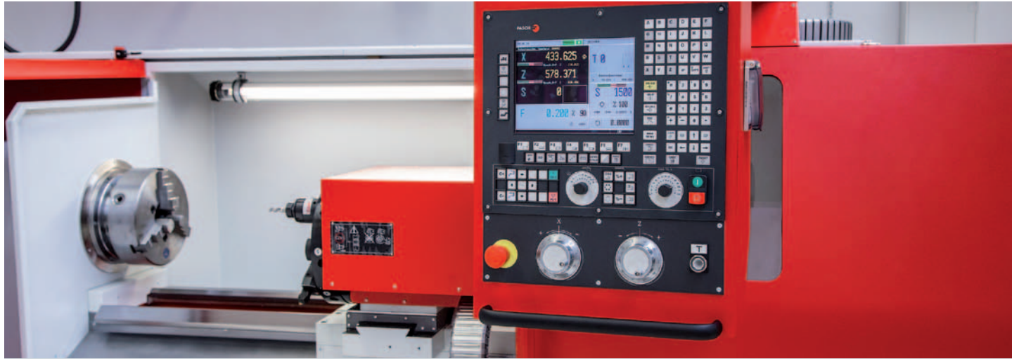
The development and design of the CNC 8055 POWER targets both operators without extensive programming skills, as well as programming specialists with extensive knowledge of ISO code. The Fagor supports dialogue programming for very simple, intuitive input with the help of defined cycles. Intuitive access keys quickly provide links to variable cycles and functions. Each individual function and each cycle can be accessed via its own access key.
