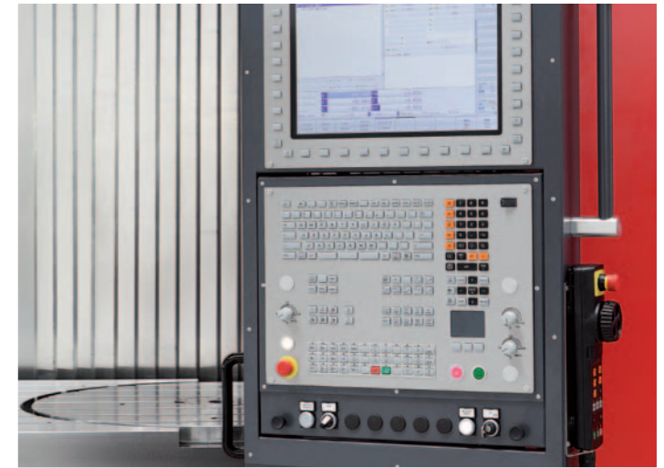
Control unit. The operator panel can travel and also rotate in the direction of the work space. This ergonomic design provides ideal working conditions for the operator.
