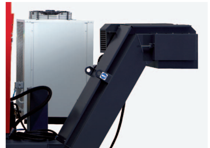
Hinge type conveyor. The chip rinsing system washes chips into the hinge type conveyor, which then automatically transports the chips from the machine into the customer provided container.
