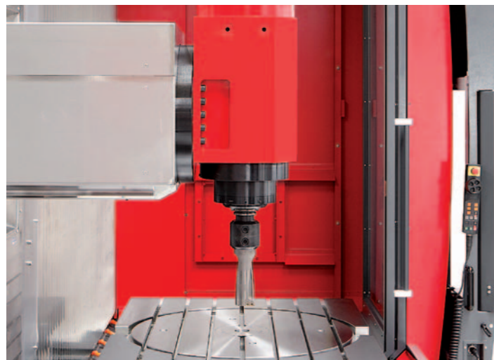
Y-axis. The Y-axis has a ram configuration. This design uses long way guides in order to attain the required rigidity.
