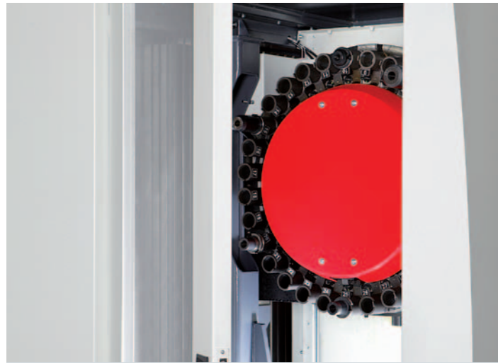
Tool magazine. Drum configuration with dual arm grippers for fast tool changes within 2 seconds. Random tool management reduces tool changing times to a minimum. Thanks to the lateral magazine door (2x in case of pendulum machining), it is possible to check and set up the tools in parallel with the machining process.
