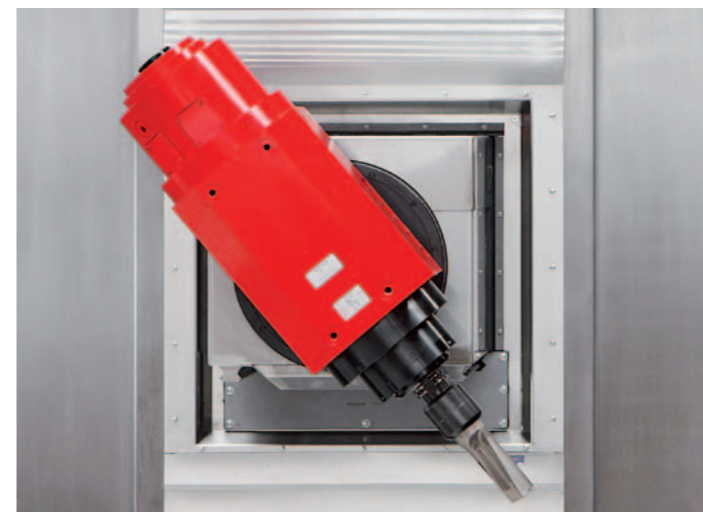
B-axis. The B-axis is driven by a torque motor, therefore achieving highly dynamic axis travel within the pivoting range of +/- 120 degrees.
