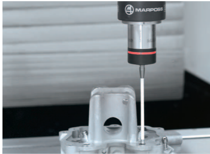
Measurement systems. Tools measurements to reduce setup times during tool changes, as well as work piece measurements to verify dimensions or to find zero locations. The work piece measurement is radio.
