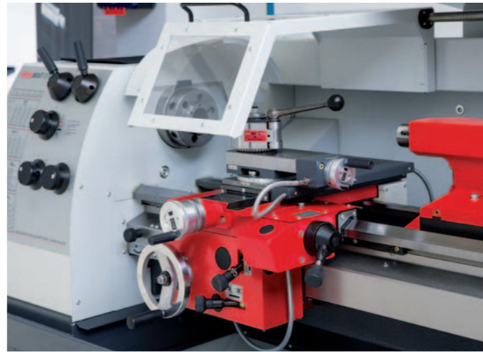
Machine design. The bed and cross slide are manually lubricated at a central point. The X and Y axes are equipped with safety hand wheels.
