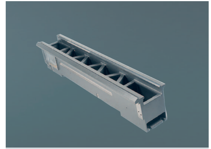
Machine bed. The machine bed's diagonal ribbing ensures optimal dropping of the chips and that the machines are rigid. The guideways are hardened and grinded. Machine bed has 3-point support.
