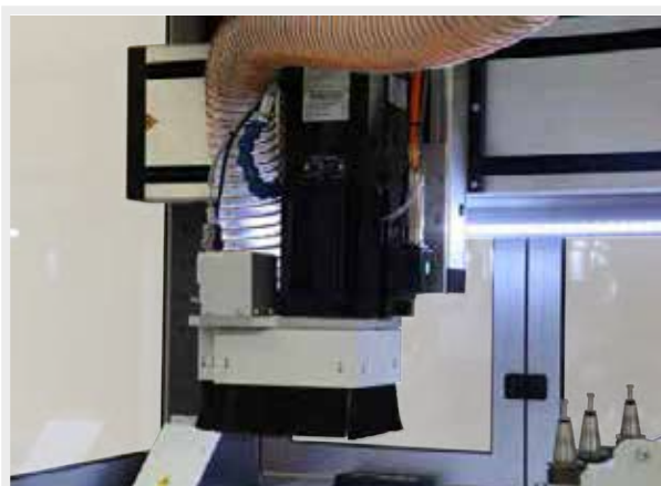
Option: suction device equipped with suction head
