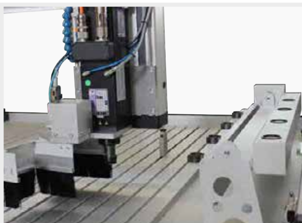
Option: automatic tool changer equipped with suction device
