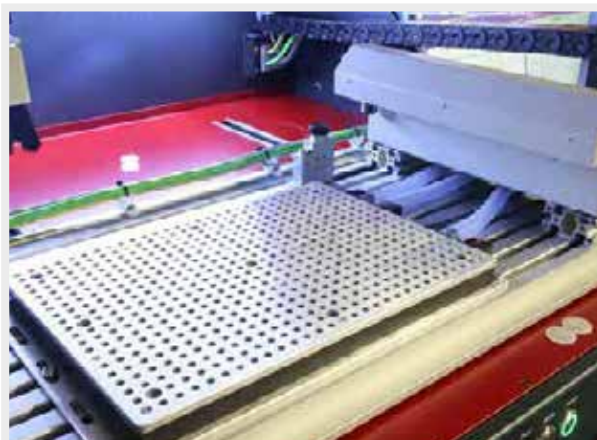
Option: vacuum clamping table and linear changer
