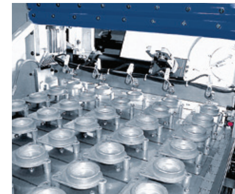
Large storage capacity chain feeding system for loading preformed blanks with the correct orientation.
