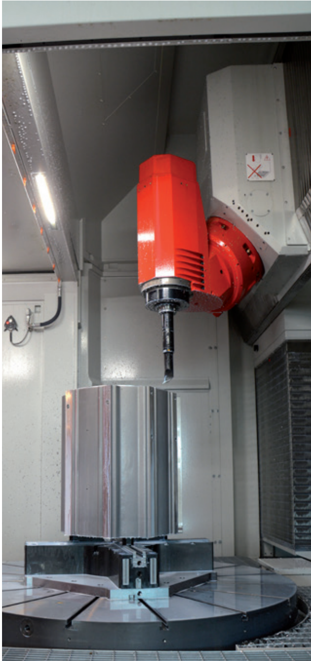
View of the work area of EMC0's Umill 1800, a 5-axis milling and turning machine used by Schwarz Elektromotoren: Reaching rotational speeds of up to 250 min -1 , the NC rotary table is able to machine components in the same way as a vertical lathe. The component shown in the picture is the biggest electric motor housing built by Schwarz so far.
